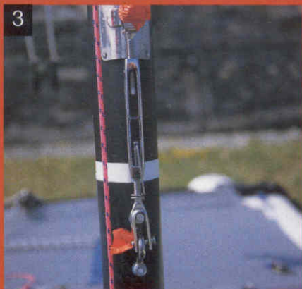
3, The diamond adjuster needs to be wound up until pre-bend in the mast matches luff curve in the sail. 4, The plastic covered trapeze loops are easy to hook onto. 5, The mouth of the chute is moulded in aluminium and glass and it fits neatly behind the main beam.
