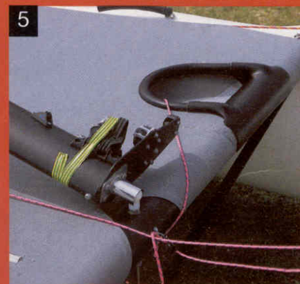
3, The diamond adjuster needs to be wound up until pre-bend in the mast matches luff curve in the sail. 4, The plastic covered trapeze loops are easy to hook onto. 5, The mouth of the chute is moulded in aluminium and glass and it fits neatly behind the main beam.
