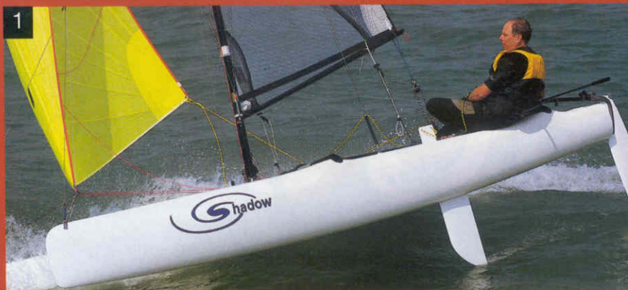
1 , Moving the bridle plates right forward allows enough room to fly a 10sq m kite inside the forestay and makes the weight, windage and clutter of a spinnaker surplus to requirements. It also means you can drop the kite on either side. 2 , Getting the mast up and down on the Shadow is a simple solo operation. The mast is virtually as light as anything in carbon and suffers from no insurance loading.
